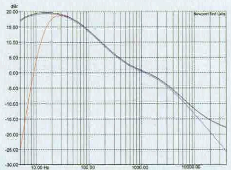
Graph 6: Phono EQ responses. RIAA Enhanced Off (blue) vs On (black); plus Rumble Filter (red).
